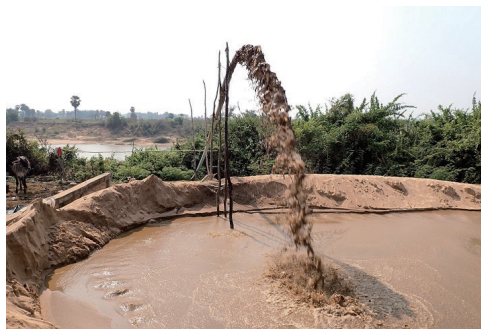
Fig.2 Sediment mining from the riverbed 図2 河床からの土砂採掘
