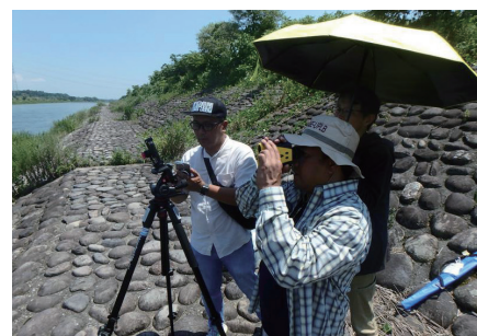
Photo 7 Participants taking a 10-second video with a cellphone to measure surface water velocity
