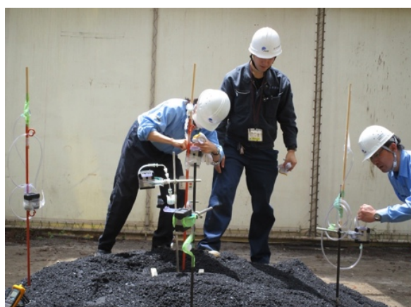
Figure 2: Measurement of asphalt fume outdoors
