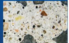
Frost attack was identified as the main cause of concrete degradation at the vicinity of the rupture plane.
