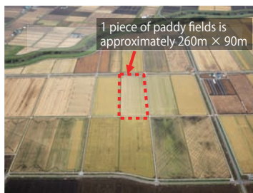
Example of large-sized paddy field after improvement: the size of 1 paddy field is about 8 times that of the traditional field.
