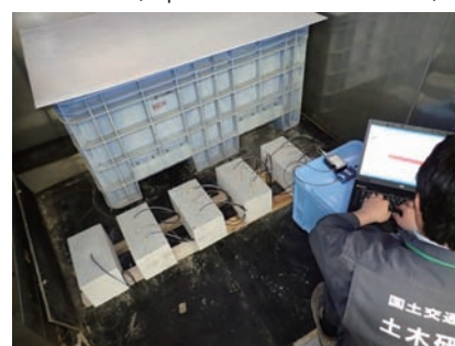
Experiment of materials having sensing functions (neutralization detection sensor)
