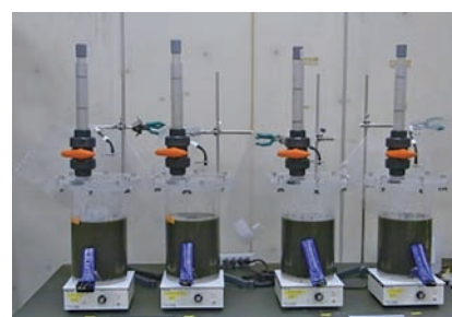
Methane fermentation experiment using a mixture of sewage sludge and crushed cut grass
