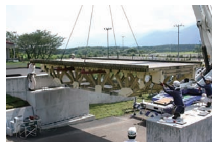
Full-scale model experiment of advanced structural materials (experiment of structural FRP)
