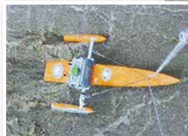
Flow rate observation technology using the ADCP
