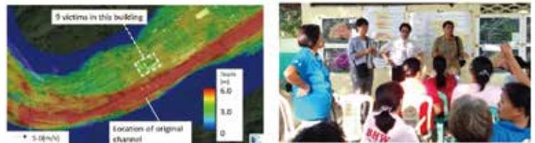
Results of the analysis of flood discharge after change in the riverbed and flow channel of a valley floor river in a semi-mountainous area
