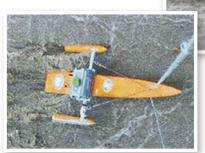
Flow rate observation technology using the ADCP
