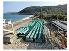
Outdoor exposure tests of concrete specimens
