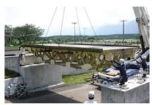
Full-scale model experiment of advanced structural materials (experiment of structural FRP)
