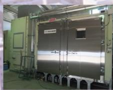
Concrete combined-deterioration accelerating test apparatus
