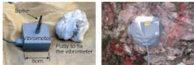
Fig. 2: Vibrometer shape and its installation
