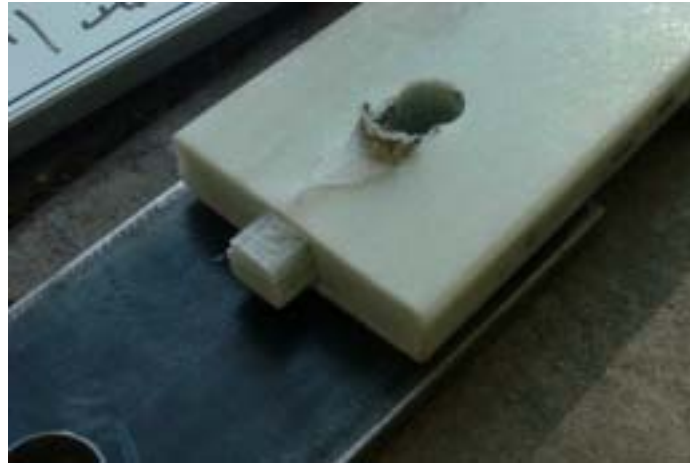
Photo.1 Specimen situation after the failure (slightly hand clamped bolt)
