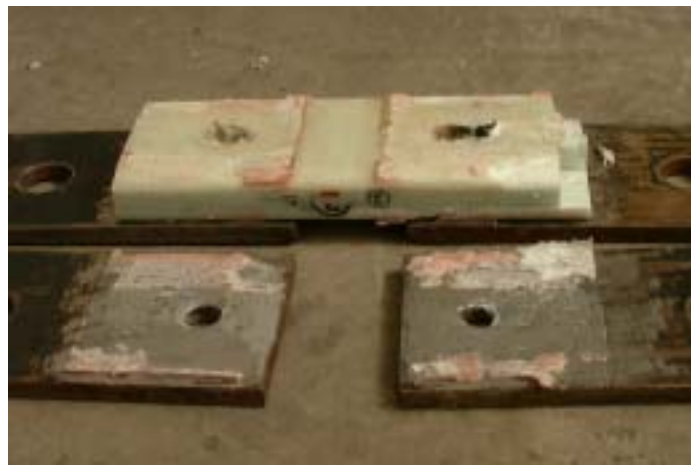
Photo.4 Specimen situation after the failure (clamped bolt and HYSOL)
