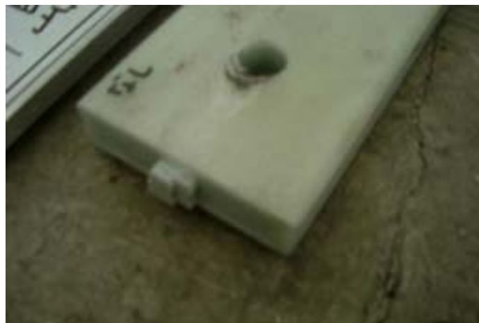
Photo.2 Specimen situation after the failure (clamped bolt)
