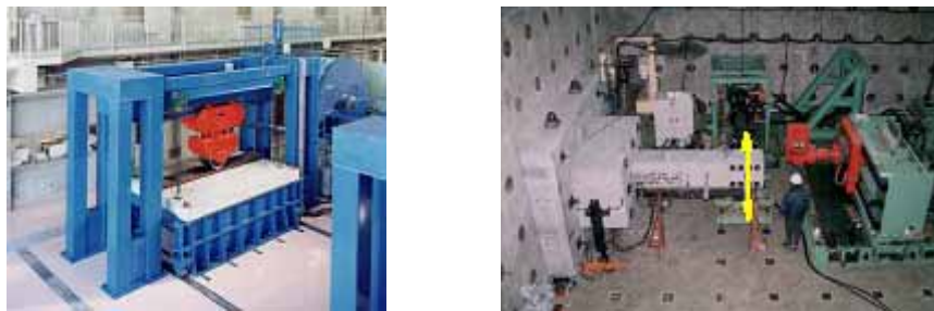
Figure 16 Tests for deck plate fatigue durability (left) and bridge pier ductility (right)
