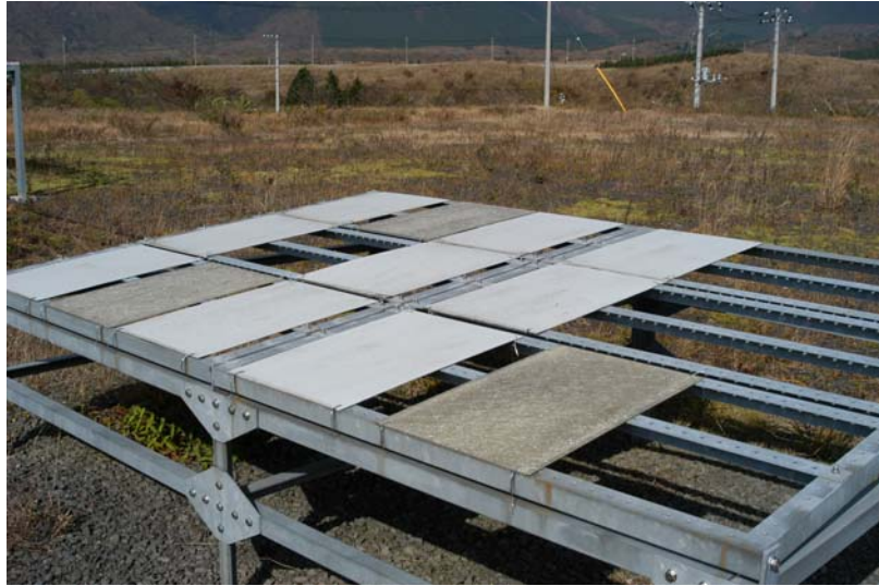
Fig. 1: Specimens under exposure test (Asagiri)
