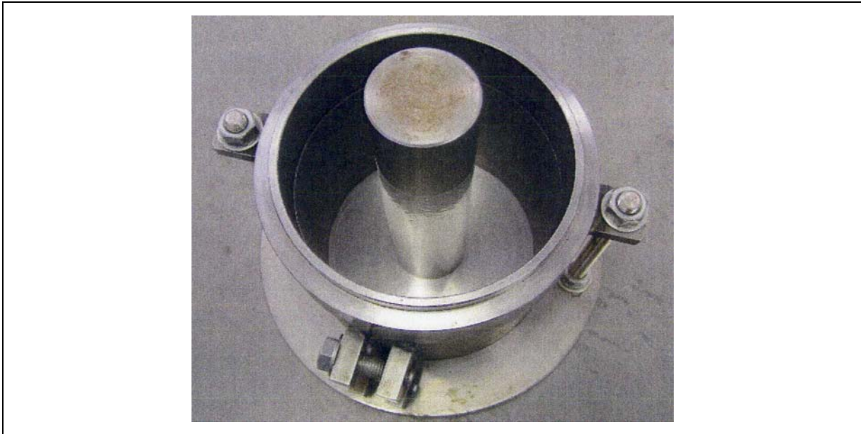
Photo 6. Mold and rod to prepare a specimen (a rod with a diameter of 5cm)
