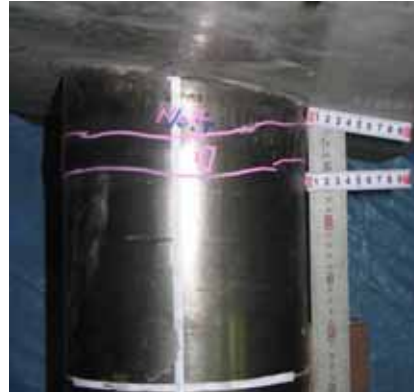
Poto.2 Final Deformation of Pile Head
