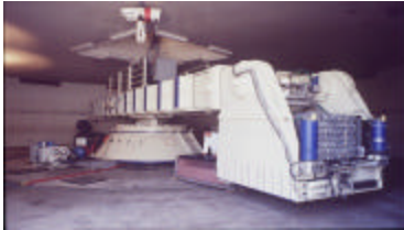
Geotechnical Centrifuge University of California, Davis
