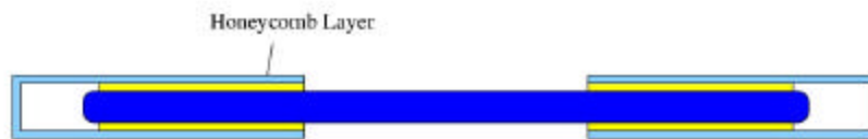
Figure 2: Polymer Matrix Composite Infill Panel (Aref and Jung, 2003)
