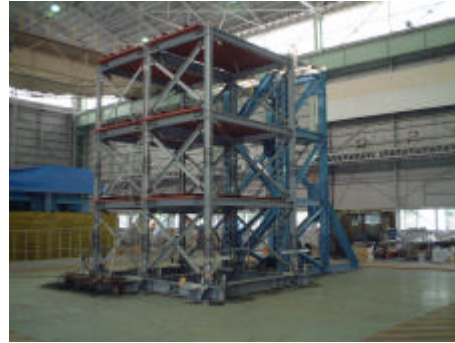
(b) Three-story test frame
