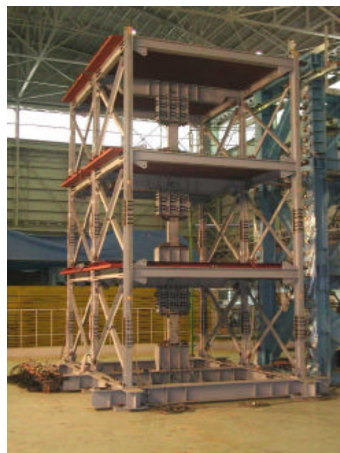
Figure 5.16 Application example - HPFRCC damper for structural control
