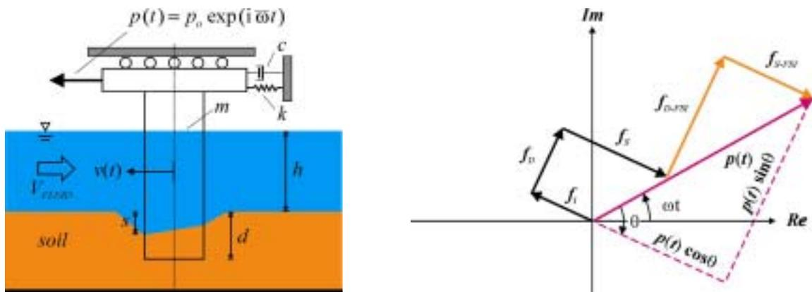
Figure 6.: SDOF system interacting with fluid and soil and closed polygon representation including additional nonlinear damping and stiffness forces
