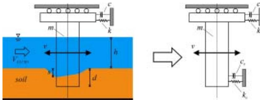
Figure 3: Equivalent fluid-soil spring-damper system
