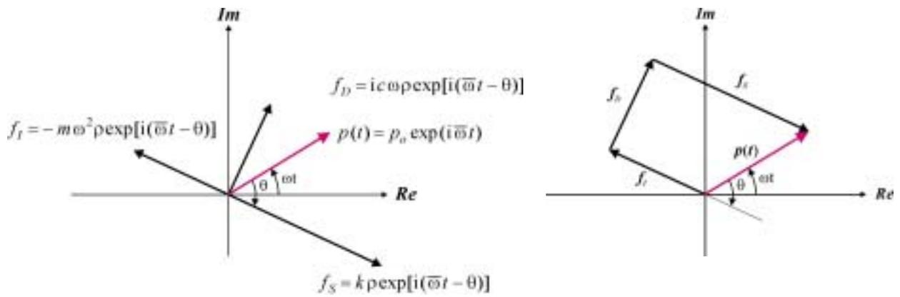
Figure 5: Steady state harmonic forces using viscous damping in a complex plane representation and closed force polygon representation
