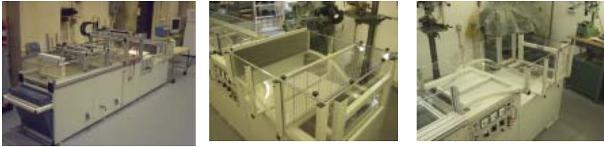
Figure 1. Test flume and trumpet shaped inlet
