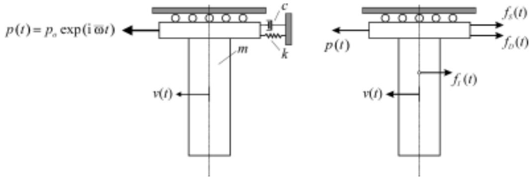
Figure 4: Linear SDOF system with basic components and forces in equilibrium
