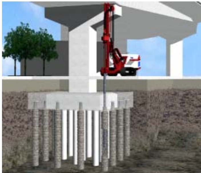
Fig.4 Micro Pile Retrofit Methods
