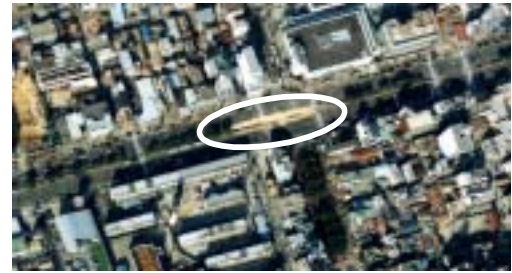
Fig-3 Subsidence at the Daikai Station (Simulated Image with 1m resolution)
