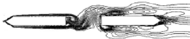
Fig.3 Flow around Slotted Box Girder
