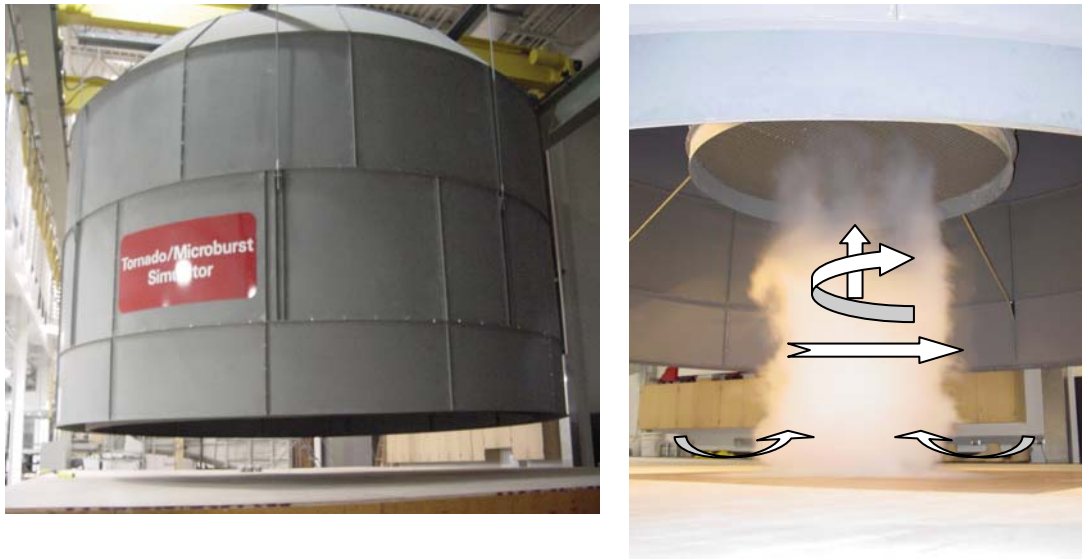
Figure 1: (a) ISU Tornado/Microburst Laboratory Simulator, (b) Flow visualization of the tornado in the Simulator showing the dynamic flow field.
