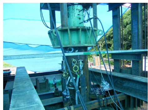
Fig.5 Setup of loading hydraulic actuator
