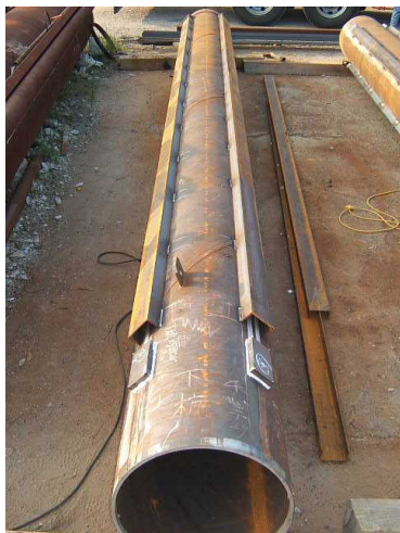
Fig. 2 Test specimen pile and attached sensors
