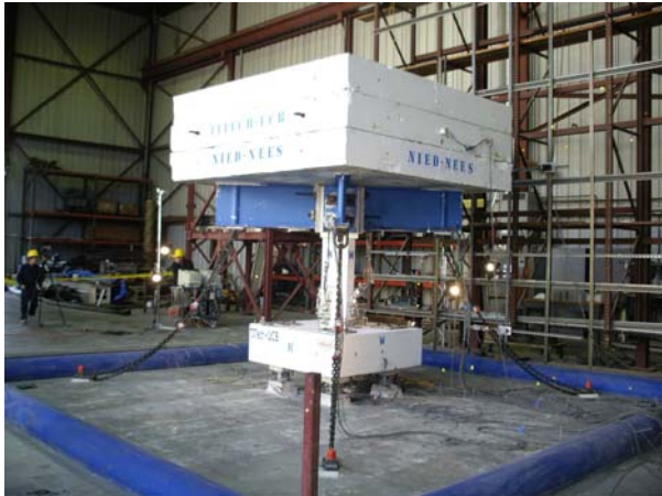
Fig. 11 Shake Table Experiment on Interlocking Spiral and Rectangular Columns (University of California, Berkeley)
