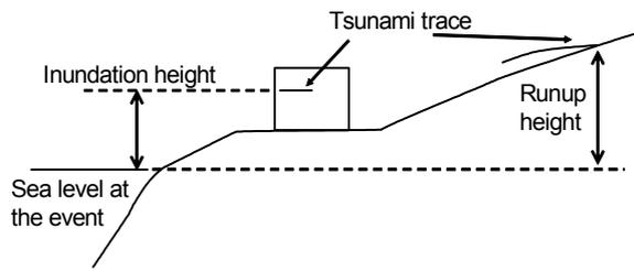
Figure 6: Definitions of inundation height and runup height
