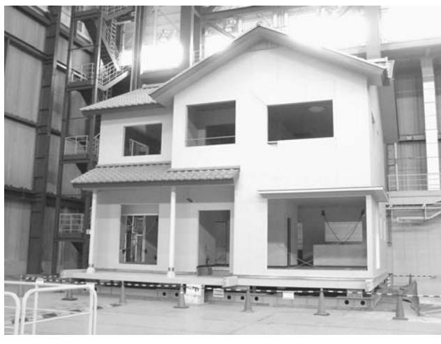
Photo of two-story typical residential house that was tested on NIED's shake table. Photo taken by S. Yim
