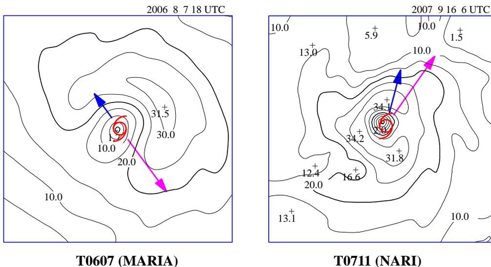
Figure 2: Isotachs for near-surface winds of Typhoons MARIA in 2006 (left) and NARI in 2007 (right) along with shear vector (pink-colored arrow) and storm motion (blue arrow).
