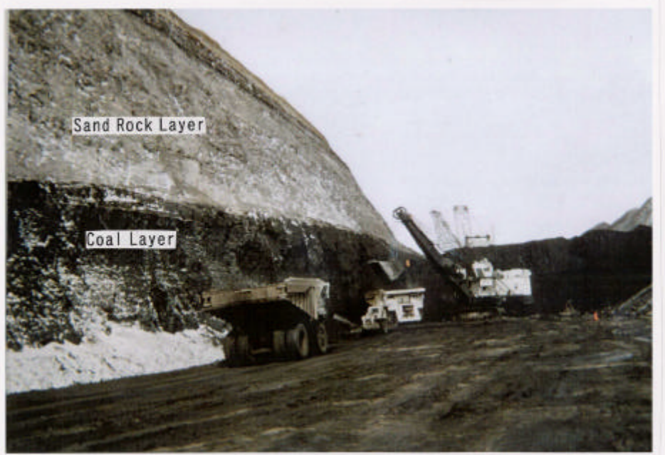
Fig. 4 : A Picture of A Surface Coal Mine (Coal is Mined by Blasting).
