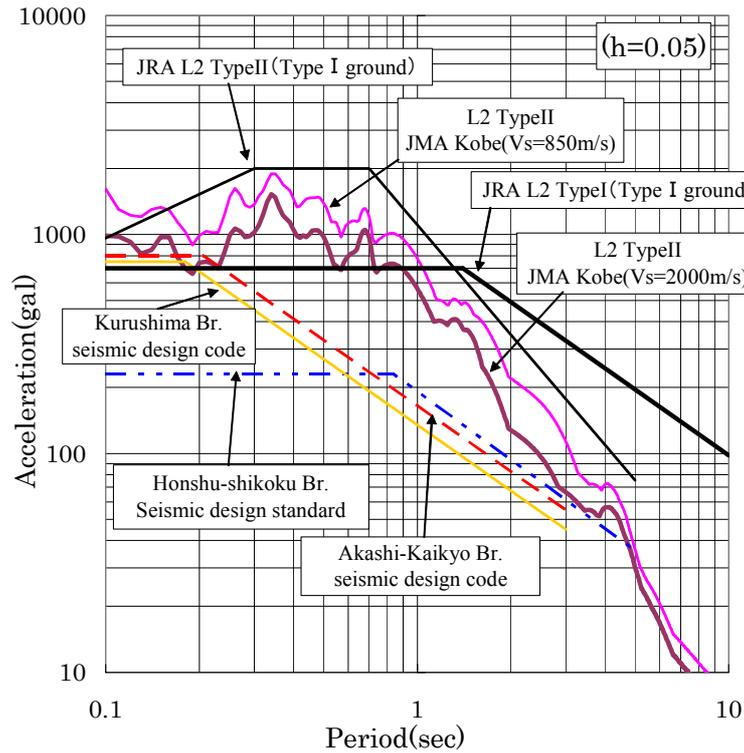
Figure2 Comparison of acceleration of each standard
