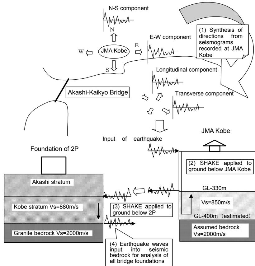
Figure4 Calculation of Earthquake Wave Input into Seismic Bedrock
