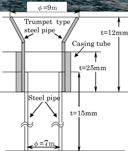
Figure7 Structure of 9m diameter column of multi-column foundation
