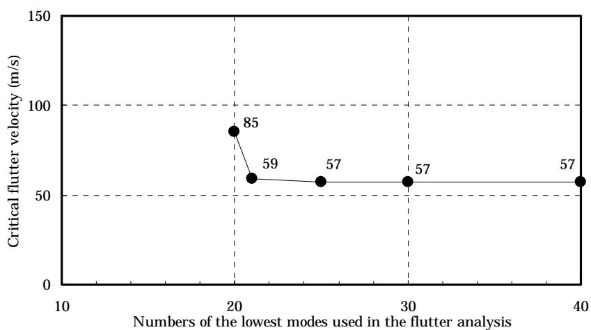
Fig.8 Influence of the lowest natural modes (Bridge-A: angle of attack=+3 deg.)
