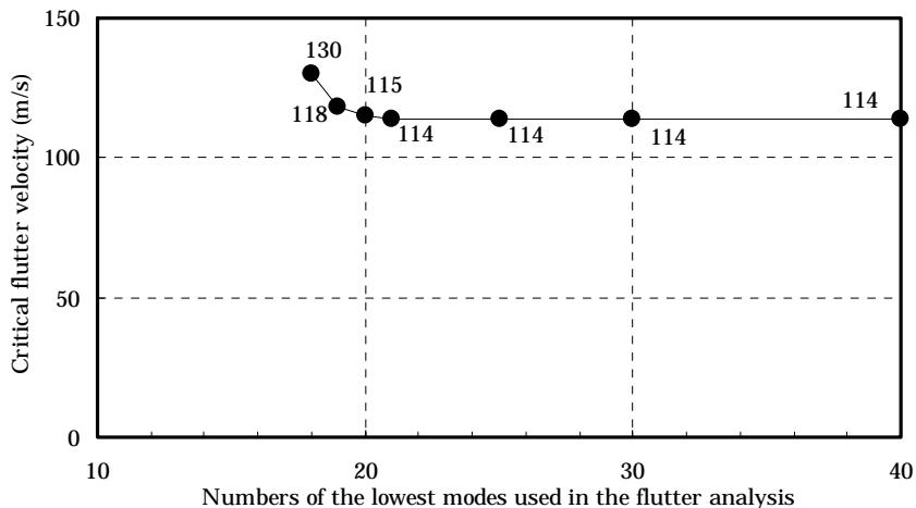
Fig.11 Influence of the lowest natural modes (Bridge-B: angle of attack=0 deg.)
