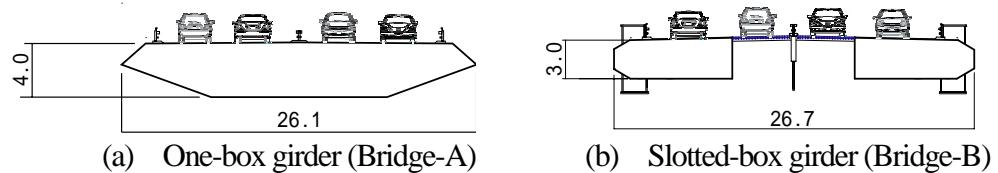
Fig.4 Cross sections of girders for four lanes (Unit: m)
