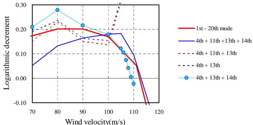
Fig.12 Selection of dominant modes (Bridge-B: angle of attack=0 deg.)
