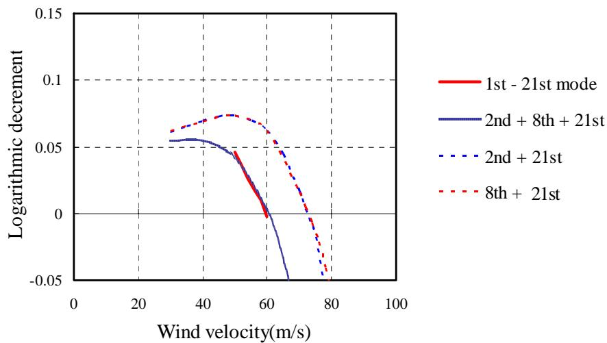
Fig.9 Selection of dominant modes (Bridge-A: angle of attack=+3 deg.)
