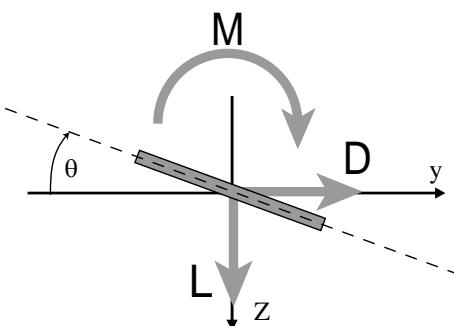
Fig.6 Coordinate system for unsteady aerodynamic forces
