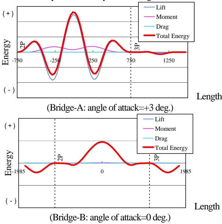
Fig.14 Spanwise distribution of energy
