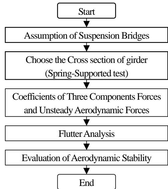
Fig.2 Procedure of flutter analysis
