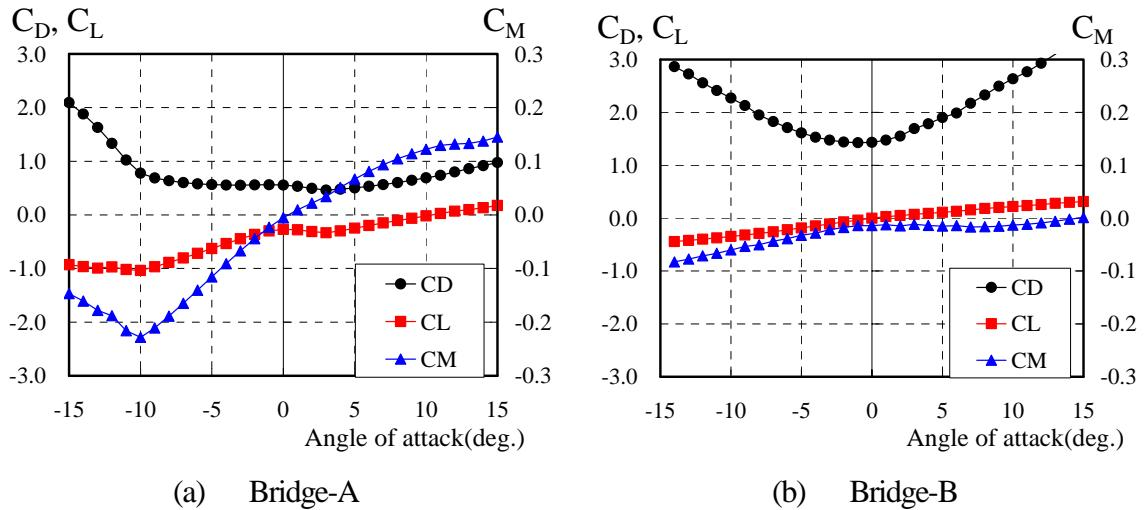
Fig.5 Coefficients of Drag, Lift and Moment
