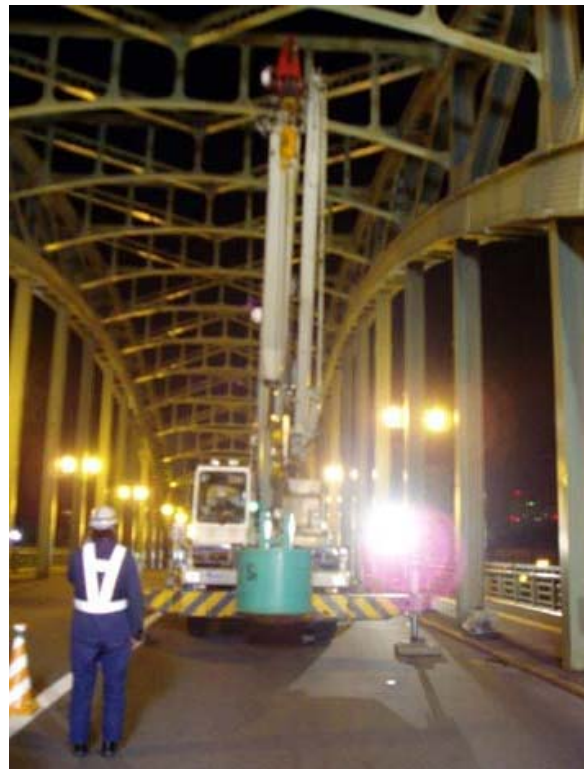
Photo 2 Forced vibration test on the bridge
