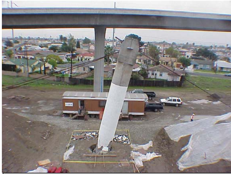
FIGURE 1 - SIX-FOOT DIAMETER COLUMN/SHAFT TEST AT UCLA.
