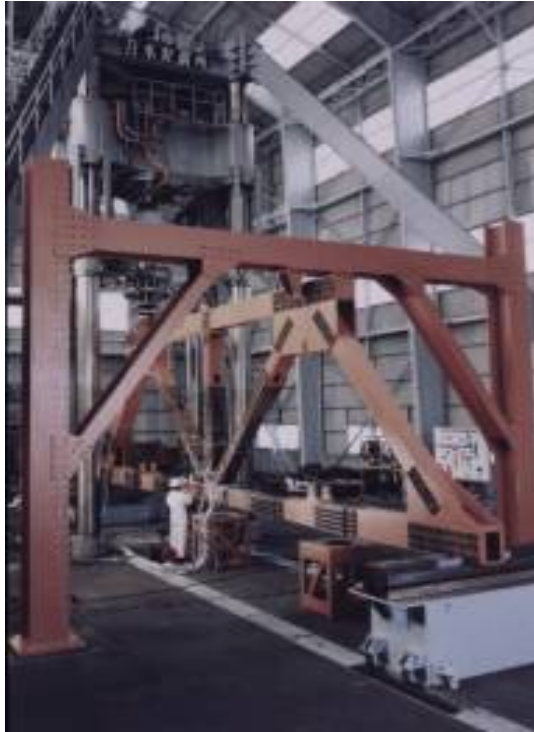
Photo 1: Fatigue test with full-scale specimen of Honshu-Shikoku Bridges
