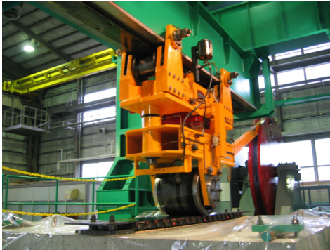
Photo 1 Wheel loading test machine
