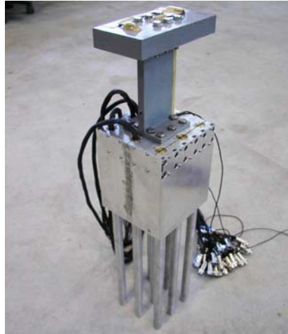
Photo.1. Model piled bridge pier with sheet pile walls (Case3-1)
