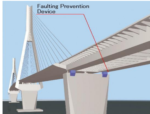
Figure-13 Faulting Prevention Device (Tsurumi Tsubasa Bridge)
