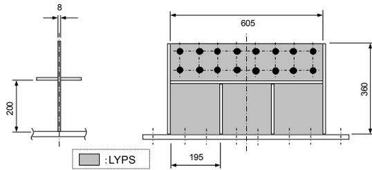
**Fig. 15** The specimen of the verification test
