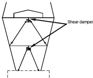
**Fig. 10** The spring modeling of shear dampers
