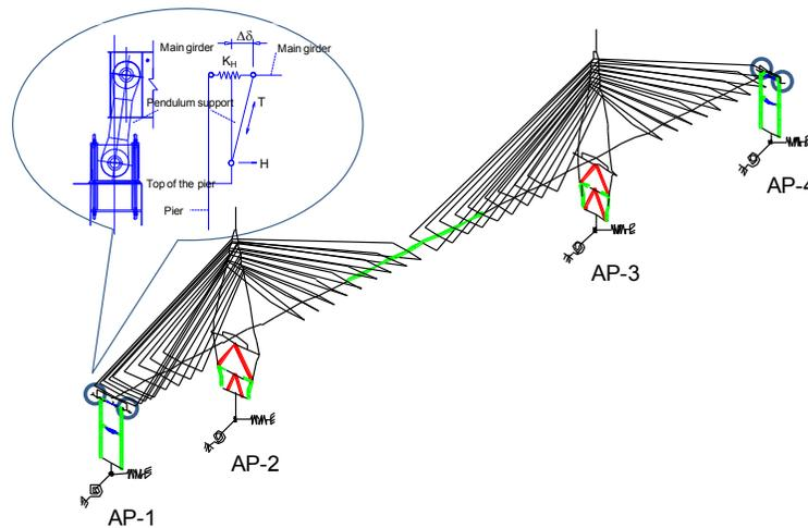
**Fig. 4** Dynamic analysis model for whole bridge
