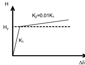
**Fig. 11** Relationship between horizontal force and displacement of shear damper
