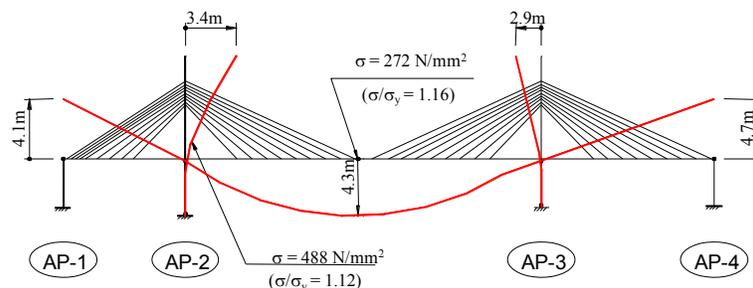
**Fig. 7** Response displacement and stress after destroying the pendulum support
