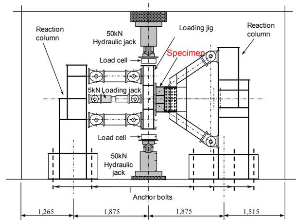
**Fig. 16** The setup of the verification test
