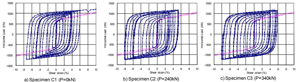
**Fig. 17** H- $\gamma$  relationship for each specimen
