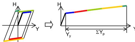
**Fig. 14** Calculation of cumulative plastic shear strain
