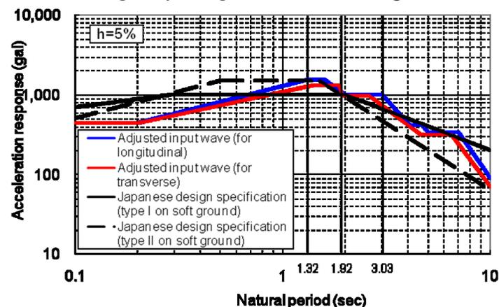
*Fig. 3* Comparison of spectral envelope and acceleration response spectrums of Japanese specifications for highway bridges
