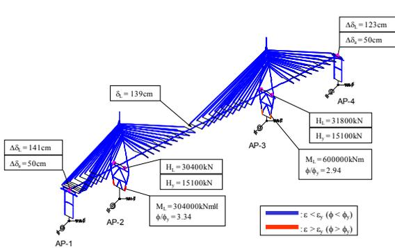
**Fig. 5** The analytical results for longitudinal response
