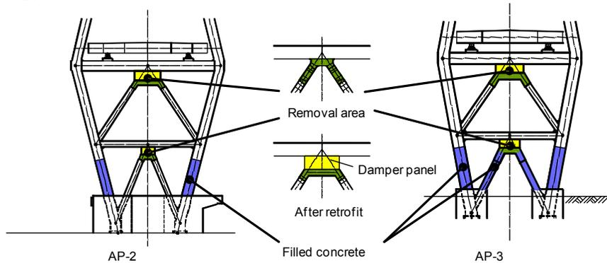
**Fig. 9** The retrofit method for the towers
