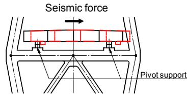
**Fig. 8** Collision between tower and main girder after destroying the pivot support
