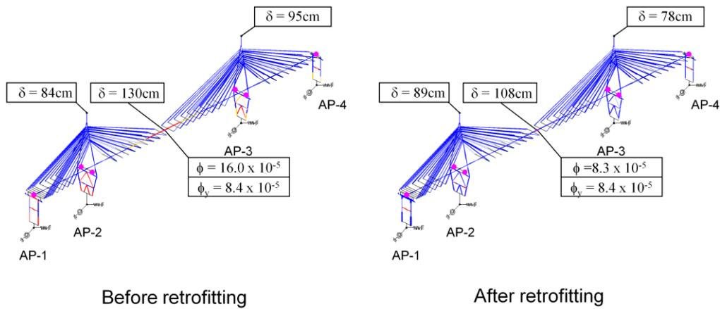
**Fig. 12** The effect of the shear dampers in seismic response
