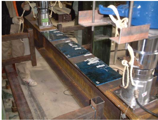
Fig.4 Test girder under loading
