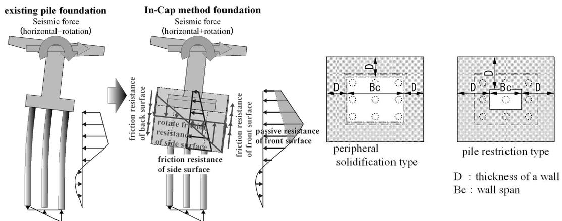
Fig. 2. Mechanism of the In-Cap method to reinforce the bearing capacity
