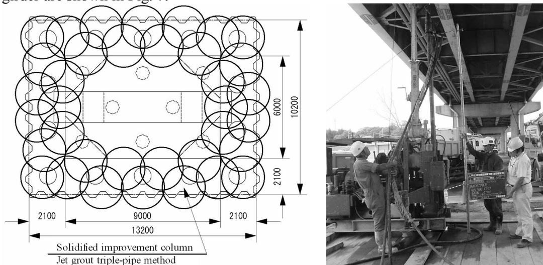
Fig. 7. Example of solidified improvement body arrangement and the actual improvement work under the girder
