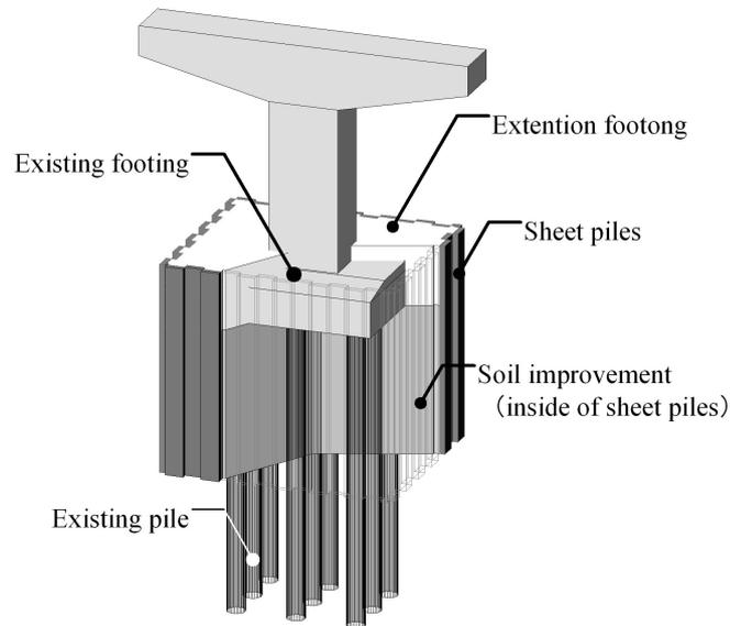
Fig. 1. Outline of reinforcing method for the existing foundation (In-Cap method)
