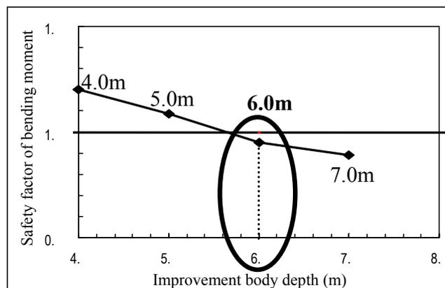
Fig. 5. Penetration depth of the solidified improvement bodies
