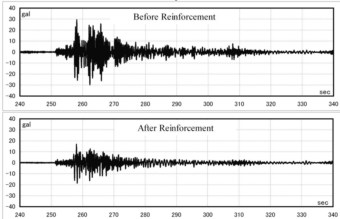
Fig. 8. Acceleration of seismic waves at the bridge piers before and after reinforcement
