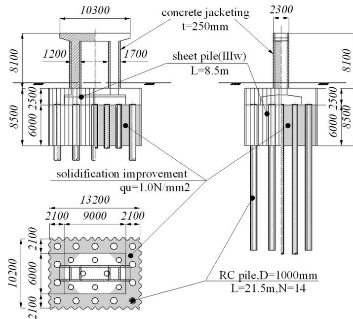
Fig. 4. Structural reinforcement diagram
