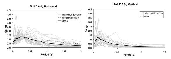
Figure 3 –Spectra of the horizontal component of ground motions scaled to match the ARS curve (Magnitude 8.0, PGA 0.5 g and site class D) at fundamental longitudinal period of base configuration, and corresponding vertical spectra
