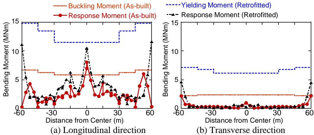
**Figure 7 Maximum response moment at arch rib**
