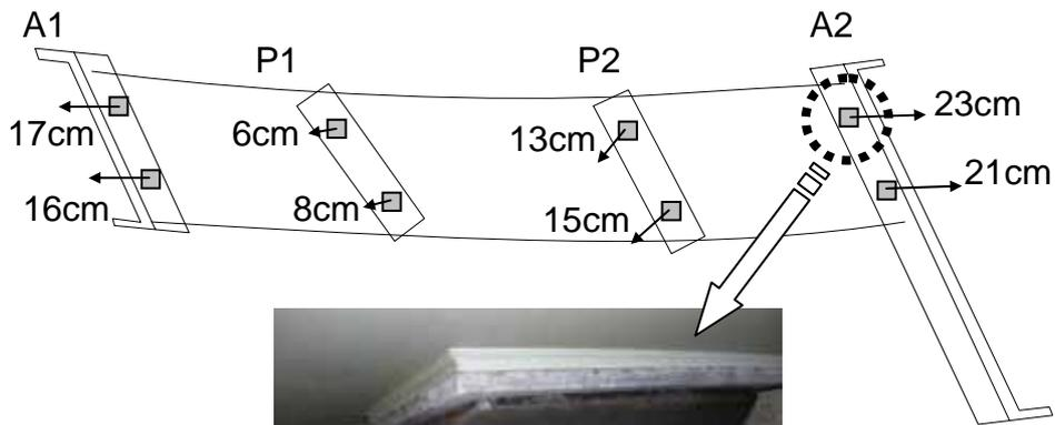
**Fig. 5** Residual displacement of rubber bearings
