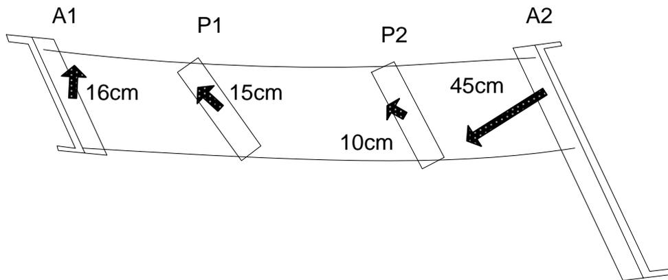
**Fig. 4** Horizontal movement of A1, P1, P2 and A2
