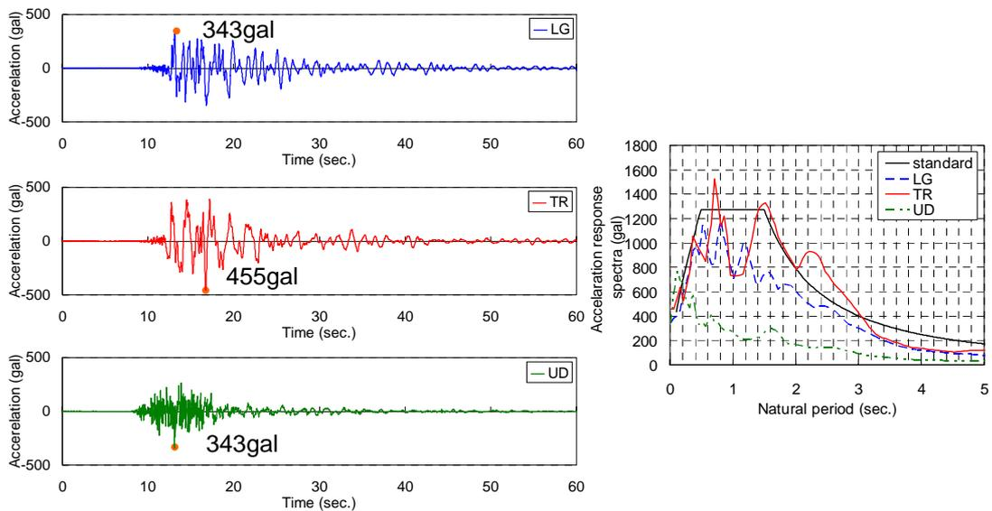
**Fig. 7 Input accelerations and acceleration response spectra**
