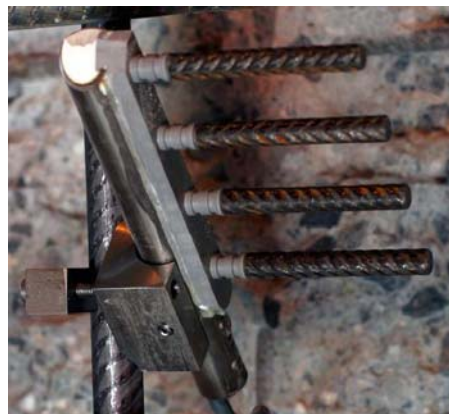
FIGURE 3: EXAMPLE OF CORSENSYS CORROSION SENSOR INSTALLATION
