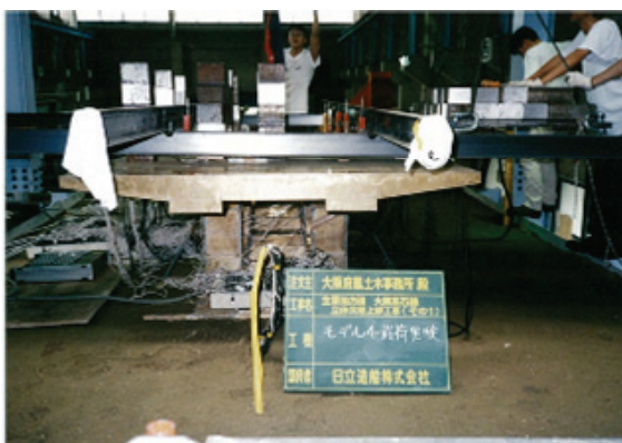
Fig. 7 Loading Test with a Scale Model
