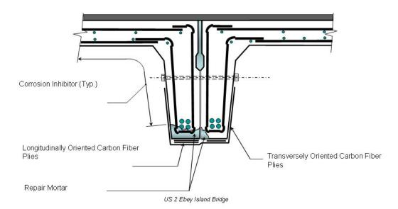
realities affect typical civil structural engineering design philosophies. The carbon fiber has an elastic modulus comparable to that of steel and an ultimate strength that is much greater than that of steel. Carbon does not possess the same ductility. This is different with respect to the traditional ductile concrete and reinforcing steel design philosophy.
