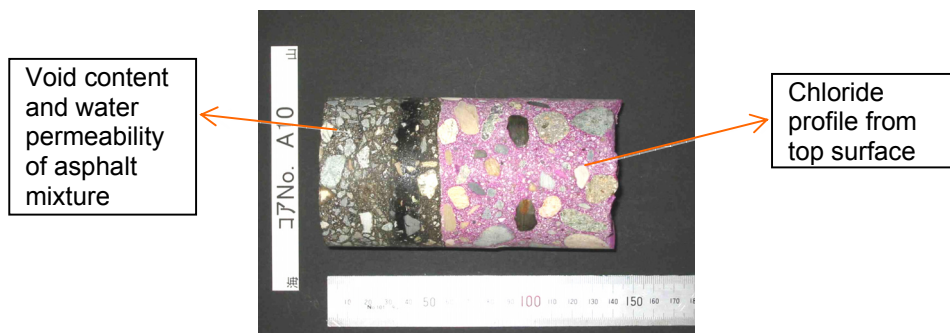
Fig. 8 A core with 70 mm dia. taken from the road surface of a closed prestressed concrete bridge at coastal area and purposes of the core
