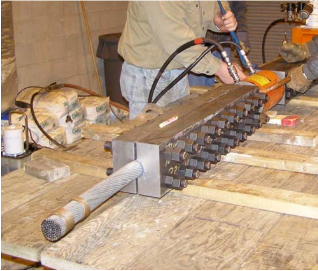
Figure 8 – Friction Clamp During Load Test
