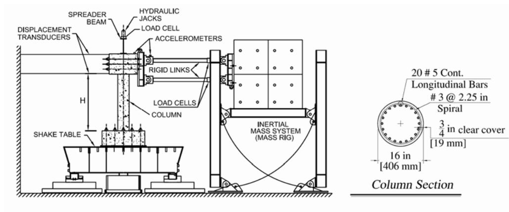
**Fig 1.** Test setup and section properties for NHS1 and NHS2
