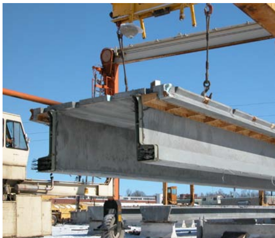
Figure 1 – UHPC Pi-girder during fabrication
